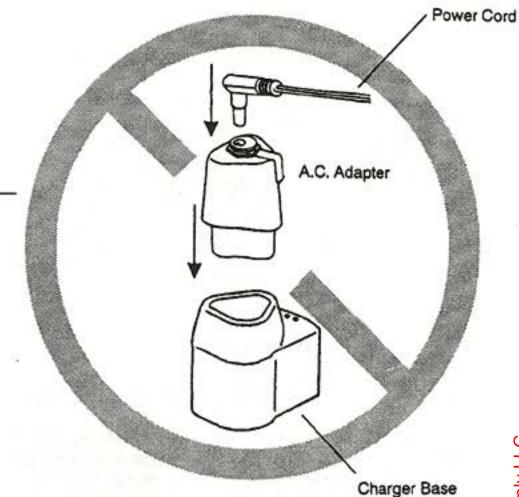
Only use A.C. Adapter to operate Scissors when using electricity.
